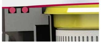
This cross section shows how the F-Neck® seals inside the filter housing
